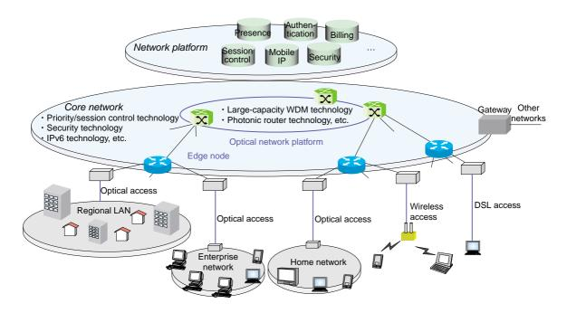
Fig. 11. Conceptual network configuration for the resonant communication environment.
