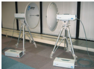
Fig. 3. Portable wireless system for digital video transmission (prototype).
