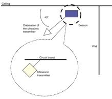
Fig. 4. Correct alignment of Cricket ultrasonic transmitter.
