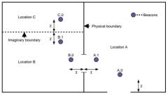
Fig. 2. Correct positioning of beacons.
