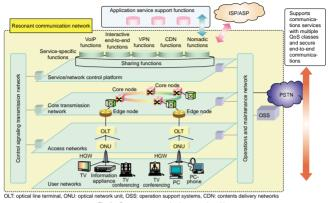
Fig. 2. Resonant communication network architecture.
