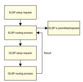
Fig. 7. Flow diagram of multi-layer routing.
