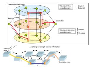
Fig. 3. Approach based on routing protocol.
