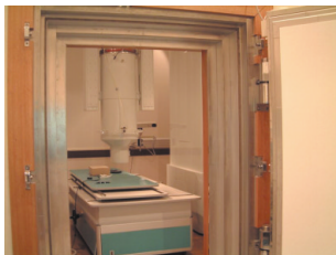
Fig. 4. External appearance of the SQUID biomagnetic measuring system (seen from the entrance to the magnetically shielded room, the middle cylindrical object is the dewar).
