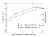
Fig. 8. MSL/slot transition characteristics versus metal thickness.
