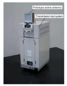
(b) Transmission test system using active integrated antenna
