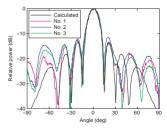
Fig. 4. Horizontal-plane radiation pattern of tested active integrated antennas.
