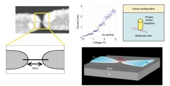
Overview of the nano-gap electrode (gap distance: 10nm)
