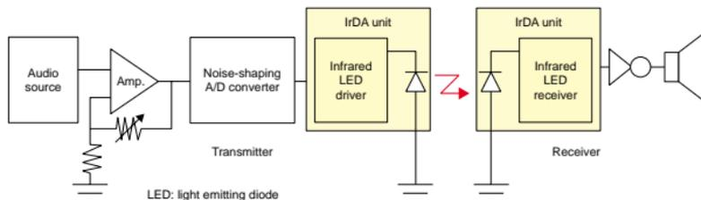
Fig. 3. *VoiceUbique* circuit block diagram.
