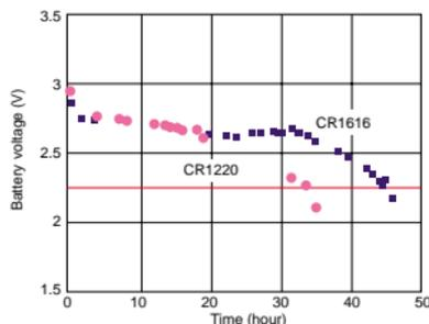
Fig. 4. Continued usage time vs. battery voltage.
