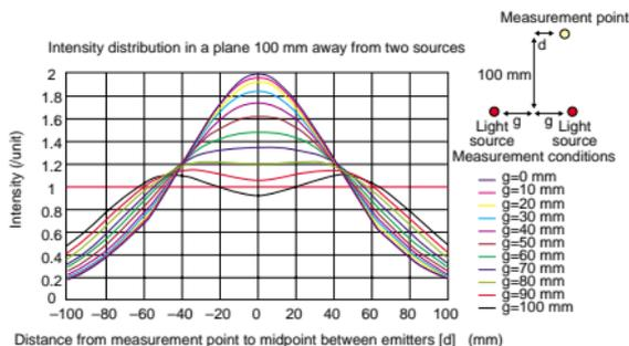
Fig. 6. Light intensity as a function of distance between units.
