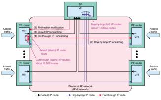
Fig. 9. Cut-through IP forwarding technology.
