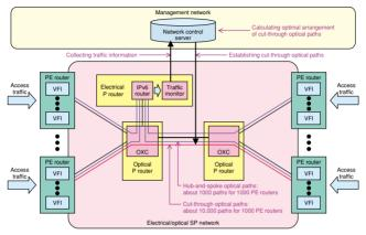
Fig. 8. Cut-through optical path control technology.
