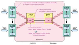
DWDM link: dense wavelength division multiplexing link, OXC: optical cross-connect
