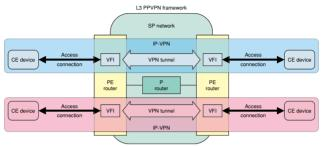
L3: layer 3, PPVPN: provider provisioned virtual private network, IP: Internet protocol, VPN: virtual private network, VFI: VPN forwarding instance, P router: provider router, PE router: provider edge router, CE device: customer edge device, SP network: service provider network
