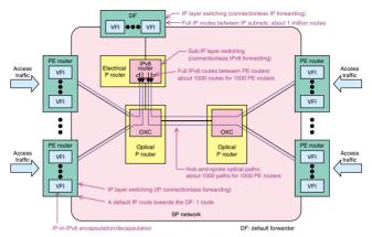
Fig. 7. IP-in-IPv6 overlay networking technology.
