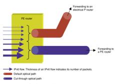
Fig. 3. Mapping IPv6 flows to optical paths.
