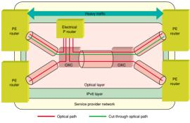
PE router: provider edge router, P router: provider router, OXC: optical cross connect
