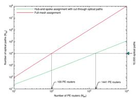
Fig. 6. Comparison of the number of optical paths.
