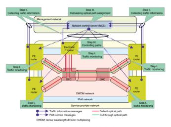
Fig. 4. Operations of cut-through optical path assignment.
