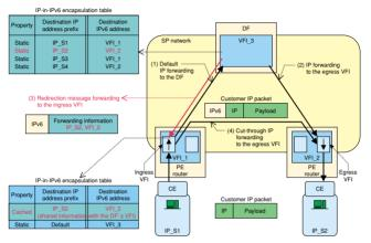
Fig. 3. Redirection control scheme.
