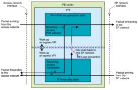
Fig. 2. Packet forwarding scheme in a VFI.
