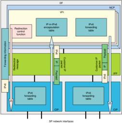
CIP: core interface package, NCP: node control package, IFP: internal forwarding package
