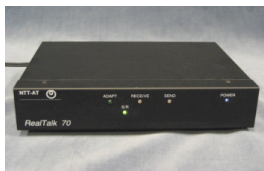
(b) Echo canceller with noise reduction unit: RealTalk 70 (NTT Advanced Technology Corp.)
