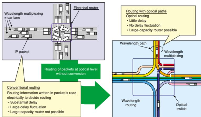
Fig. 7. Routing with optical paths.
