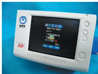
3-D imaging volume: 4 inches diagonally and 5 mm deep
