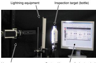
Line-sensor camera Captured image on display terminal (expanded image of all sides)
