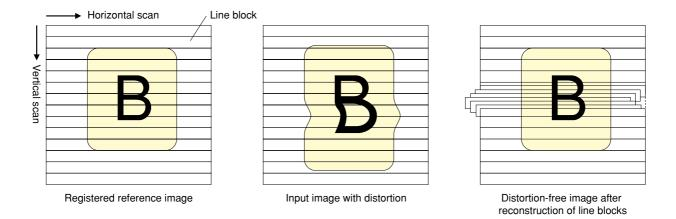
Fig. 3. Line-block distortion reduction method for pattern-matching inspection.
