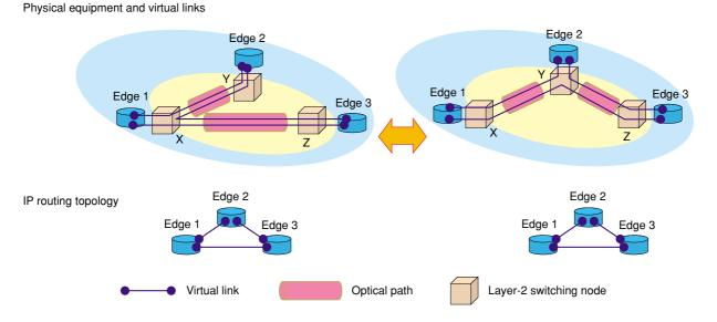
Fig. 6. Optical path cut-through with virtual links.
