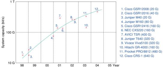
Fig. 1. Router performance versus commercial introduction date.
