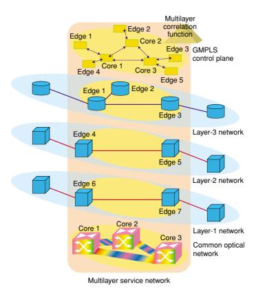
Fig. 4. Example network architecture for multilayer service network.
