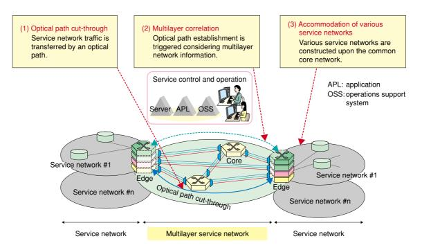
Fig. 2. Network architecture for multilayer service network.
