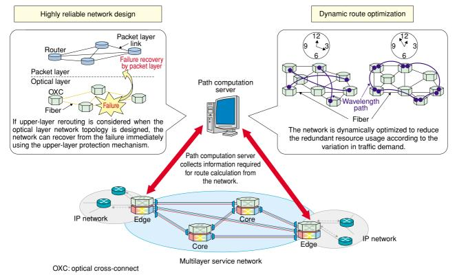
Fig. 4. Example of a network providing advanced traffic engineering.
