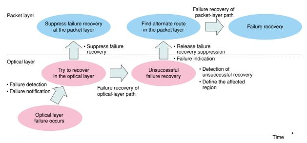
Fig. 3. Failure recovery through multilayer coordination.
