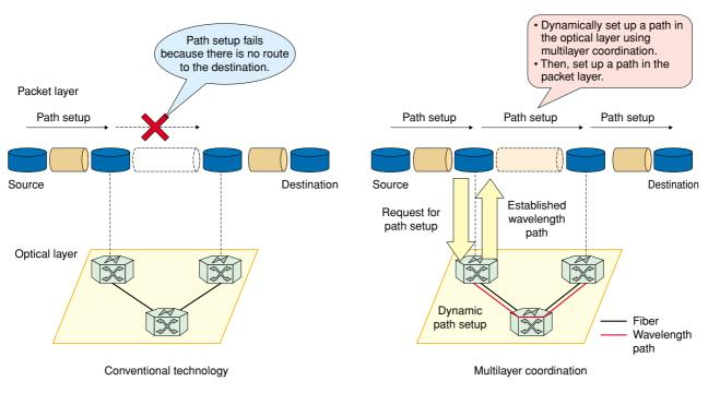
Fig. 2. Dynamic path control achieved by multilayer coordination function.
