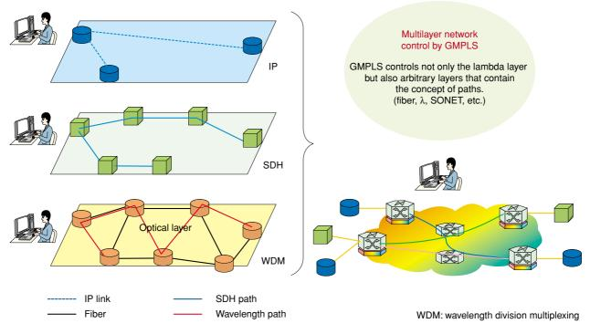
Fig. 1. Concept of multilayer network control.
