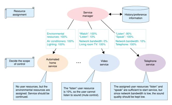
Fig. 3. Service control and autonomous decision of scope of control according to resource assignment.
