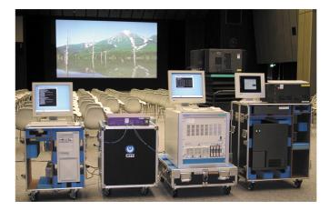
Fig. 1. SHD digital cinema distribution system. From the left: PC-server, GbE-hub, JPEG2Krealtime decoder and projector (GbE: gigabit Ethernet).
