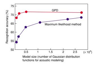
Fig. 2. This figure illustrates that GPD consistently produces higher recognition rates than its traditional counterpart, the maximum likelihood method, in an example word recognition task.
