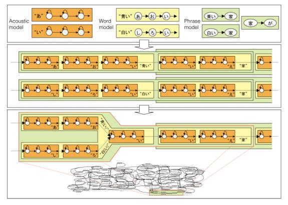
Fig. 3. This figure illustrates the behavior of the finite-state transducer that is currently studied at NTT Communication Science Laboratories for large vocabulary speech recognition.
