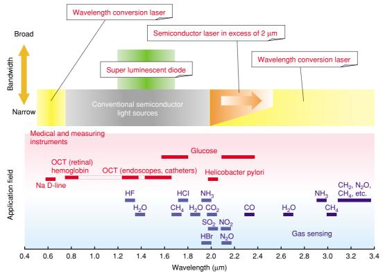
Fig. 1. Application fields and bandwidths of the new light sources.
