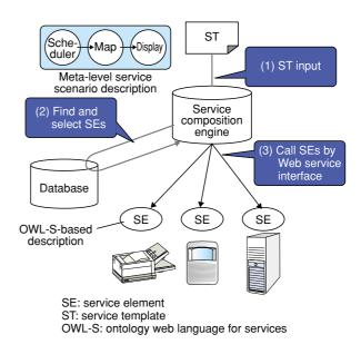
Fig. 3. Basic mechanism of service composition.
