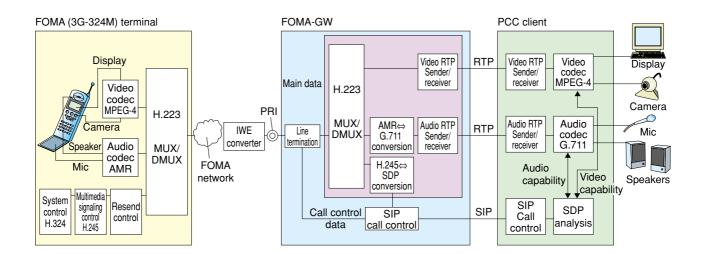
H.324: ITU-T Recommendation. A multimedia communication system that uses the analog telephone network. 3G-324M is a specification that is based on the H.324 mobile network version H.324/M.
