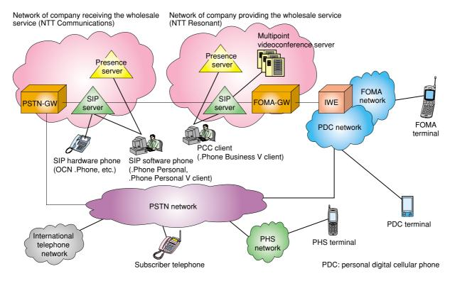
Fig. 1. PCC system and network configuration.
