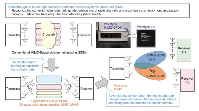
Fig. 1. Multi-user MIMO for future high-capacity wireless system.
