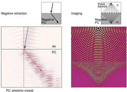
Fig. 3. Negative refraction in photonic crystals.
