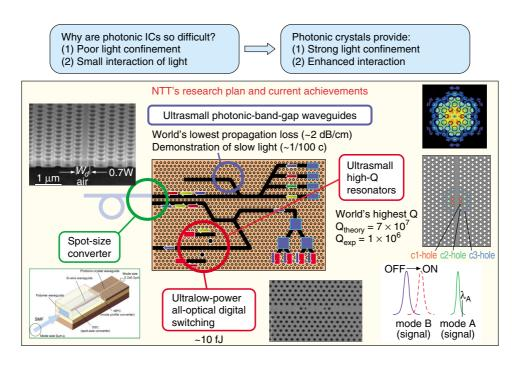
Fig. 2. Photonic integrated circuits on photonic-crystal platform.
