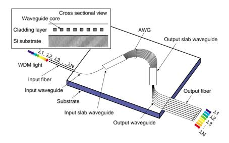
Fig. 1. AWG-type wavelength multiplexer/demultiplexer using PLC. Input light is demultiplexed into different outputs thank to the prism-like dispersion function of the AWG.
