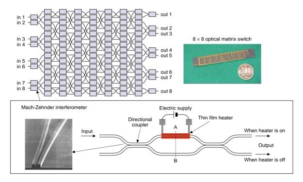
Fig. 3. Structure of a Mach-Zehnder-interferometer optical switch (8 × 8). The device divides input light along two optical waveguides and switches the output port according to the phase difference between the two signals after merging. A phase difference is generated by changing the temperature of a waveguide using a heater (on/off operation). Integrating a large number of these switches (as shown by the matrix switch in the upper left) leads to large-scale switching.
