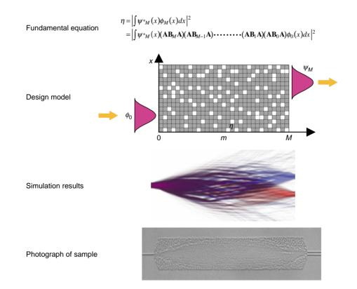
Fig. 2. Generation of waveguide pattern by wavefront matching method. A waveguide pattern is automatically designed by inverse-calculation for maximum η. The pattern shown in the picture can separate 1.3- and 1.5-μm lights.
