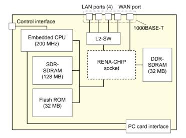
Fig. 3. Configuration of RENA-CHIP evaluation board.
