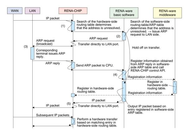
Fig. 4. Example of RENA-ware operation (ARP table registration).
