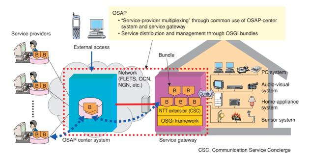
Fig. 3. Outline of OSGi Service Aggregation Platform (OSAP) (using home services as an example).
