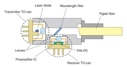
Fig. 2. Bi-directional optical transceiver.
