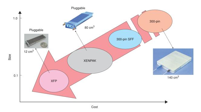
Fig. 1. MSAs of 10-Gbit/s optical transceivers.
