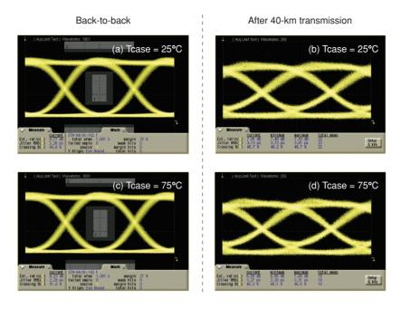
Fig. 3. Eye diagrams for 10.7 Gbit/s NRZ-PRBS 2<sup>31</sup>-1.
