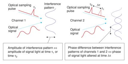
Fig. 1. Principle of linear optical sampling.
