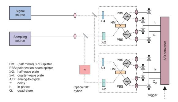
Fig. 2. Equipment configuration.
