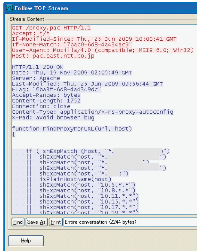
Fig. 10. Content of HTTP communications (command requests and replies).
