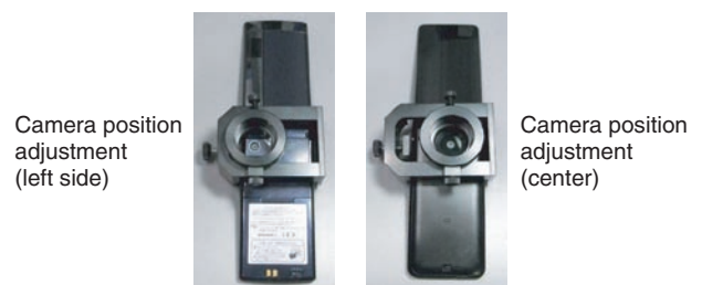
Fig. 7. Cell phone attachment.
