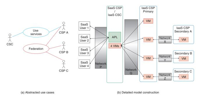
Fig. 3. Abstracted use cases and detailed model construction.
