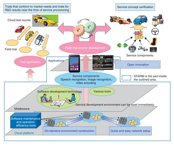
Fig. 2. Overview of XFARM configuration.
