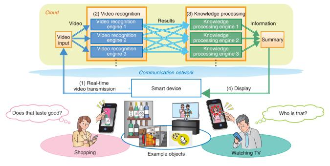
Fig. 2. Function configuration of SightX.
