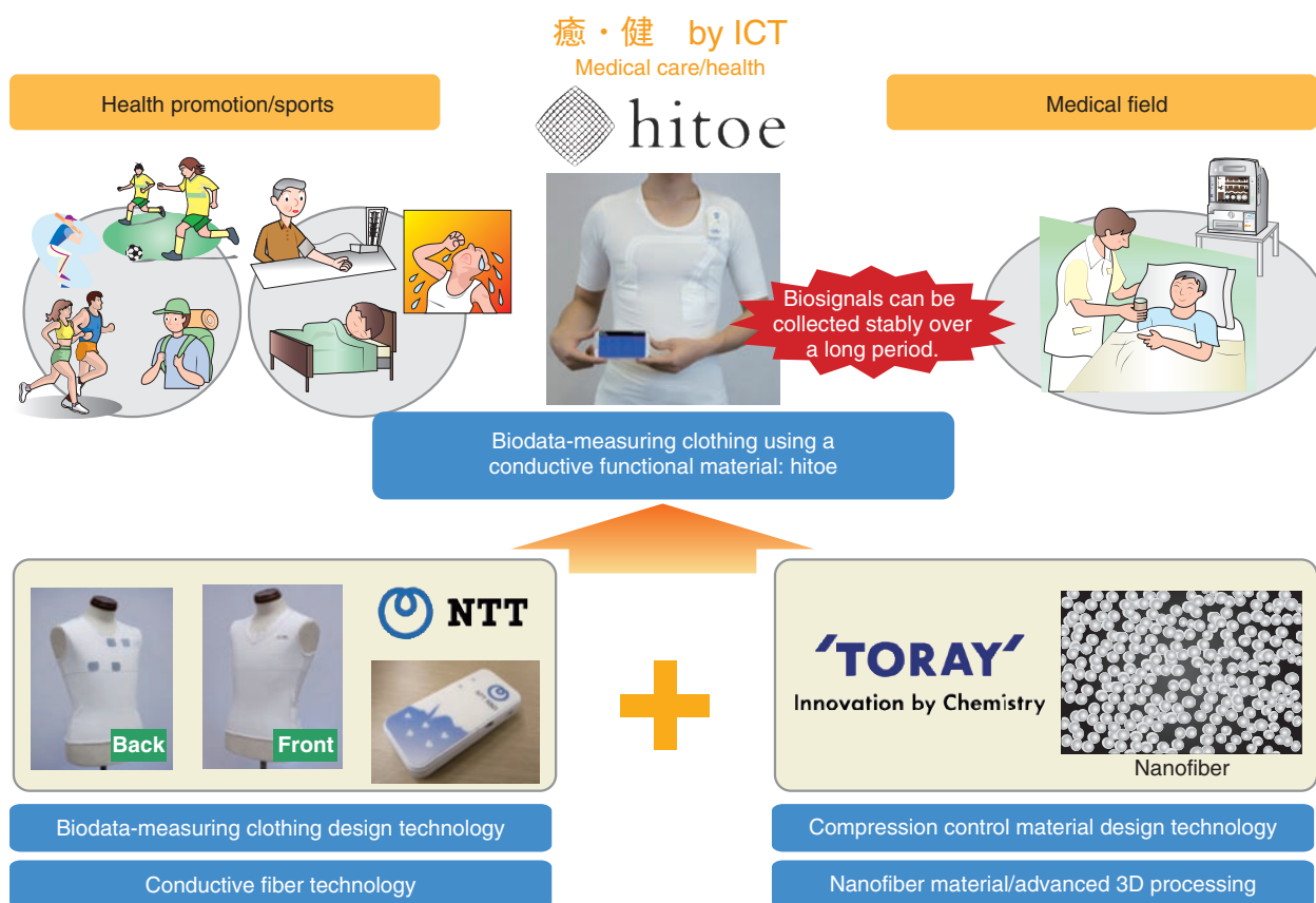
Fig. 13. Bio-electrode made of conductive polymer/fiber materials, developed with Toray.
