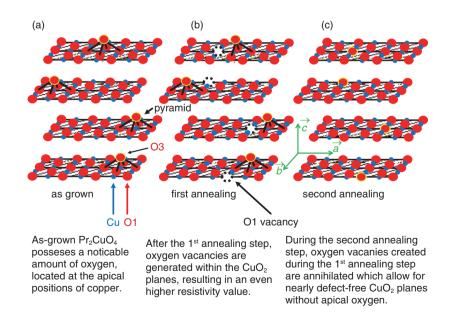
Fig. 6. Microscopic view of oxygen vacancies and defects at each synthesis or annealing step.
