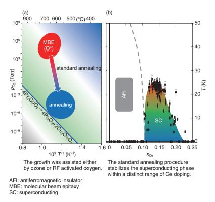
Fig. 3. (a) Thermodynamic phase diagram in the vicinity of the growth conditions of Pr<sub>2-x</sub>Ce<sub>x</sub>CuO<sub>4</sub> (red area) and annealing conditions (blue area) and (b) superconducting phase diagram of Pr<sub>2-x</sub>Ce<sub>x</sub>CuO<sub>4</sub> grown on (001) SrTiO<sub>3</sub> substrates as a result of the annealing procedure shown on the left.
