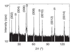
Fig. 2. X-ray diffraction pattern taken of Pr<sub>2</sub>CuO<sub>4</sub> grown on (001) SrTiO<sub>3</sub> substrate.
