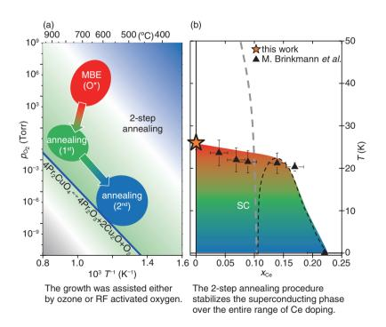
Fig. 4. (a) Thermodynamic phase diagram in the vicinity of the growth conditions of Pr<sub>2-x</sub>Ce<sub>x</sub>CuO<sub>4</sub> (red area) and annealing conditions (green and blue area) and (b) superconducting phase diagram of Pr<sub>2-x</sub>Ce<sub>x</sub>CuO<sub>4</sub> grown on (001) SrTiO<sub>3</sub> substrates as a result of the annealing procedure shown on the left. Data denoted by triangles are taken from Ref. [34].
