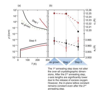
Fig. 5. (a) Temperature dependence of resistivity of Pr<sub>2</sub>CuO<sub>4</sub> thin films in as-grown state (green dashed line), after the 1<sup>st</sup> annealing step (step I), and after the 2<sup>nd</sup> annealing step (step II) and (b) trace of the crystallographic lattice parameters of Pr<sub>2</sub>CuO<sub>4</sub> thin films.
