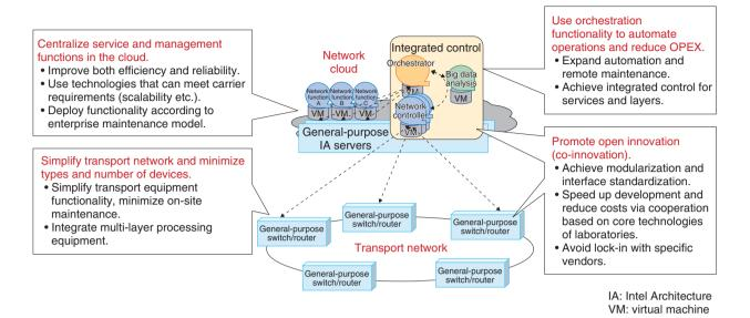
Fig. 1. Innovations of network architecture and development schemes with virtualization technologies.
