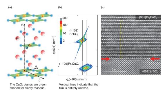
Fig. 1. (a) Crystal structure of Pr<sub>2</sub>CuO<sub>4</sub>, (b) high-resolution reciprocal space map of Pr<sub>2</sub>CuO<sub>4</sub> grown on (001) SrTiO<sub>3</sub> substrate, and (c) high-resolution transmission electron microscopy image of Pr<sub>2</sub>CuO<sub>4</sub> grown on (001) SrTiO<sub>3</sub> substrate taken at the interface.
