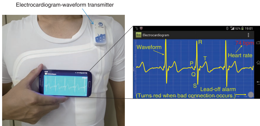
Fig. 6. Electrocardiogram measurement using smartphone.
