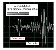
(b) Measured results for artificial defect in a buried rod
