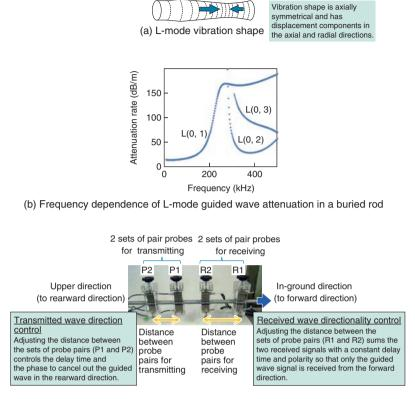
(c) Example of probe arrangement on rod
