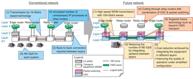
NE-OpS: network element operation system OXC: optical cross-connect
