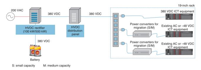
Fig. 2. HVDC power supply system configuration.
