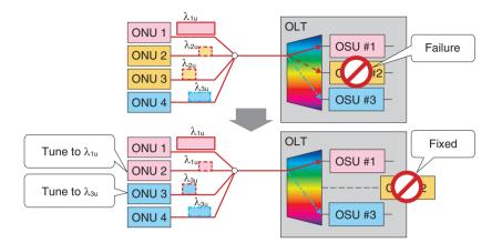
Fig. 3. Example of OLT protection technology using wavelength tuning in ONUs.
