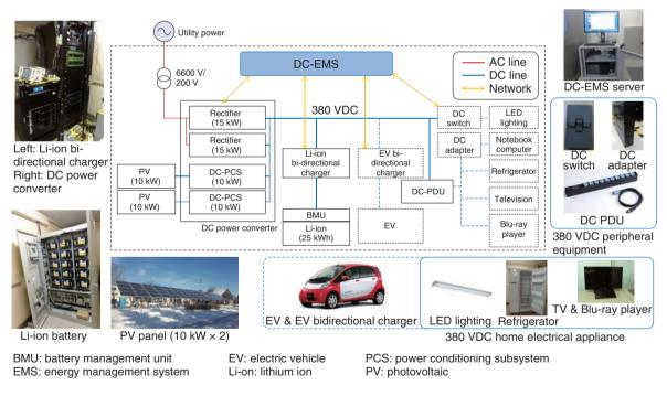
Fig. 4. Ministry of the Environment Field Testing System (Obihiro, Hokkaido).
