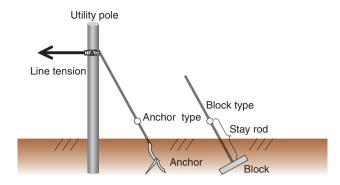
Fig. 1. Utility pole support: anchor and block types.
