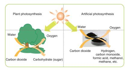
Fig. 5. Comparison of artificial and natural photosynthesis.
