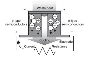
Fig. 9. Thermoelectric conversion principle.
