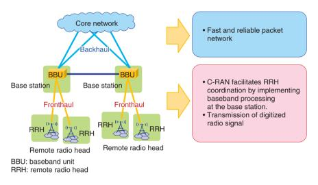
Fig. 4. Example mobile network configuration.
