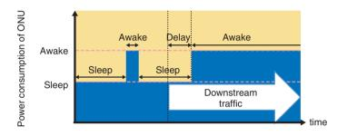
Fig. 5. Termination of TRx sleep caused by downstream traffic.
