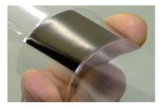
Fig. 10. Thermoelectric element (1 square inch).
