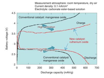
Fig. 3. Initial charge/discharge curves of lithium-air rechargeable batteries using a ruthenium oxide catalyst.
