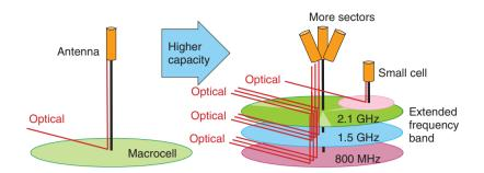
Fig. 3. Example of optical lines used with radio base station.
