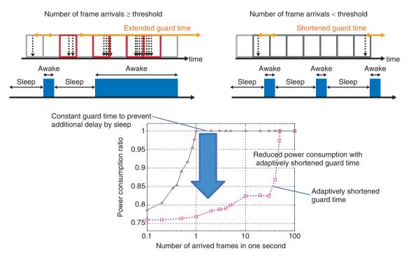
Fig. 6. Power reduction with proposed adaptive guard time control.
