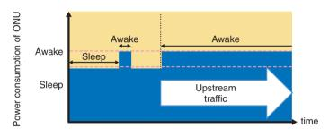
Fig. 3. Termination of Tx/TRx sleep caused by upstream traffic.
