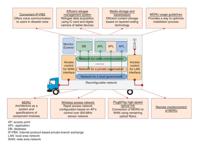
Fig. 2. Major enabling technologies applied in MDRU architecture.
