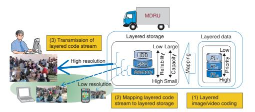
Fig. 3. Layered data transmission.
