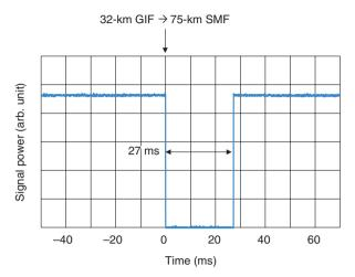
Fig. 4. Evolution of received 10GbE signal level (32-km GIF  $\rightarrow$  75-km SMF).
