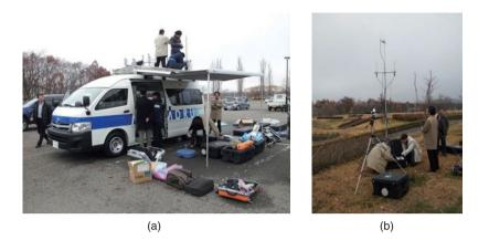
Fig. 4. MDRU installation experiment; (a) preparation for wireless module distribution, and (b) setup of Wi-Fi module.
