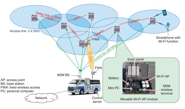
Fig. 1. Wireless access network system using M2M wireless access.
