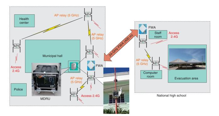
Fig. 3. MDRU and wireless equipment installed at San Remigio Municipal Hall and at a high school.
