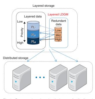
Fig. 4. Source and repair packet deployment for distributed storage.
