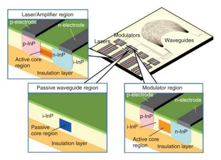
Fig. 1. Concept of PICs based on membrane optical devices.
