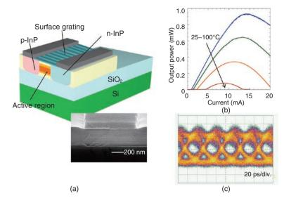
Fig. 5. (a) Device structure, (b) current-output characteristics, and (c) 25.8-Gbit/s modulating waveform of DFB laser on SiO<sub>2</sub>/Si.
