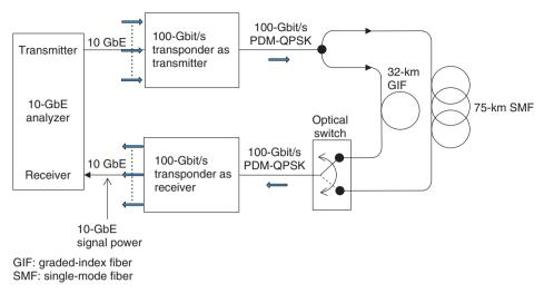
Fig. 2. Experimental setup for optical route switching of 100-Gbit/s signal.
