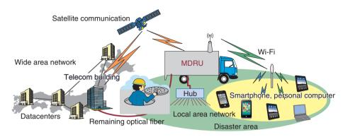
Fig. 1. Concept of MDRU architecture.
