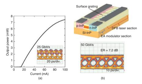
Fig. 4. Characteristics of membrane devices on InP: (a) directly modulated DFB laser, and (b) EA-DFB laser.
