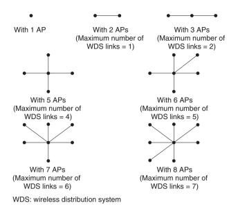
Fig. 3. Measured network topologies.
