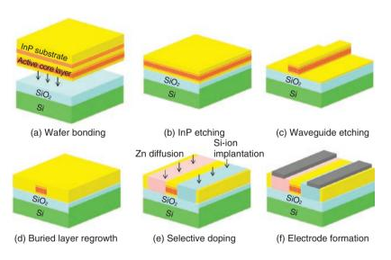
Fig. 3. PIC fabrication processes employing selective doping techniques.
