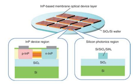
Fig. 2. Membrane optical devices integrated on silicon.
