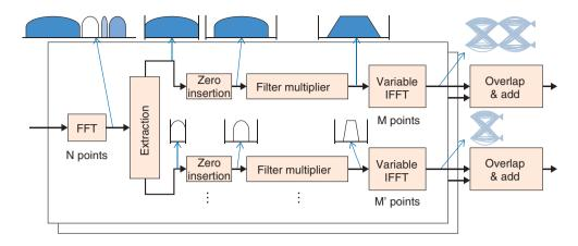
Fig. 4. Configuration of proposed multi-rate arbitrary-arrangement-type FFT filter bank (MR-FFTFB) in the receiver.
