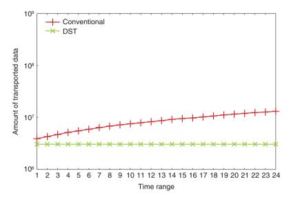
Fig. 5. Time range vs. amount of data transported in MapReduce.
