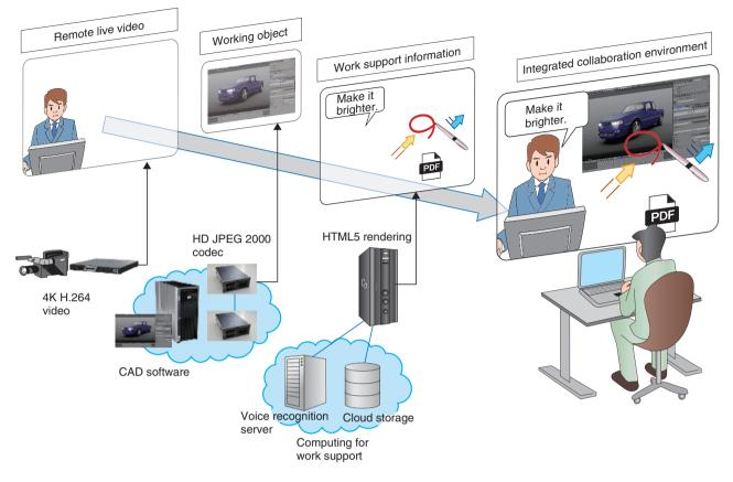
Fig. 4. Overview and application example of Augmentation Layer.
