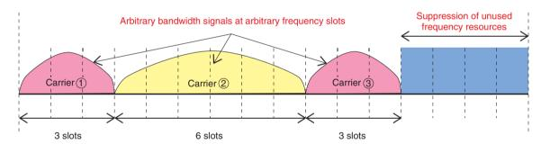
Fig. 5. Improved spectrum efficiency with HEGMM.
