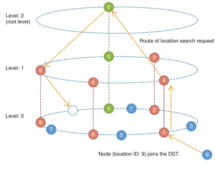
Fig. 3. Node join process in DST.
