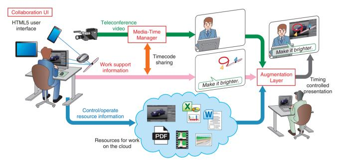
Fig. 3. Block diagram of REMOCOP.
