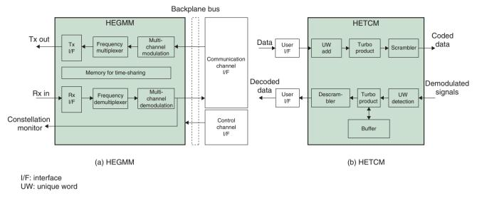
Fig. 6. Configurations of HEGMM and HETCM.
