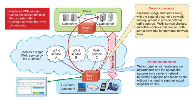
Fig. 1. Conceptual diagram of Smart CPE.
