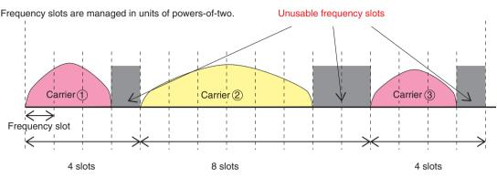
Fig. 3. Problem of unused frequency slots with GMM.
