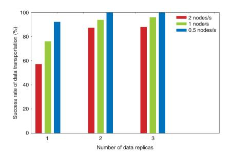
Fig. 6. Success rate of data transportation vs. the number of data replicas.
