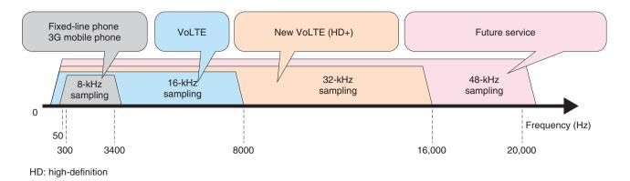
Fig. 1. Supported audio bandwidth in EVS.
