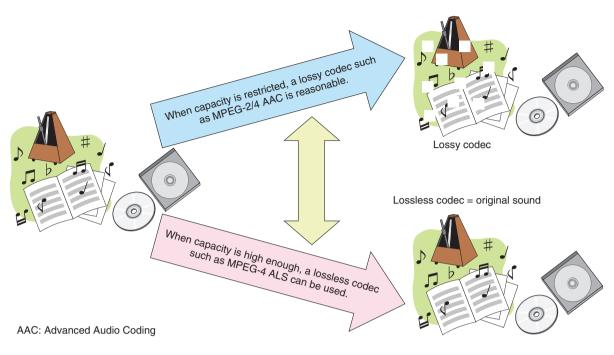
Fig. 2. Selection of audio codec according to the allowed bit rate.
