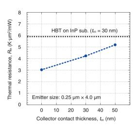
Fig. 6. Thermal resistance as a function of collector contact thicknesses of fabricated HBTs.
