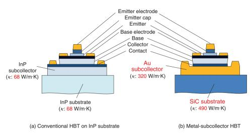
Fig. 1. Cross-sectional view of (a) conventional InP-based HBT on InP substrate and (b) metal-subcollector HBT on SiC substrate.
