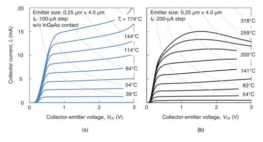
Fig. 7. *I*<sub>C</sub>-*V*<sub>CE</sub> characteristics of HBTs fabricated on (a) SiC substrate and (b) InP substrate. Dotted lines show junction temperatures estimated from *R*<sub>th</sub>.
