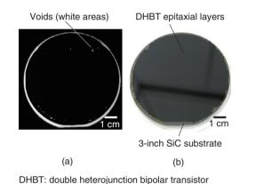
Fig. 3. (a) Scanning acoustic microscope image of HBT epitaxial layers on an InP substrate bonded to an SiC substrate. (b) Photograph of the bonded wafer after removal of InP substrate.
