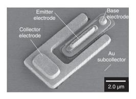
Fig. 4. Scanning electron microscope image of a fabricated metal-subcollector HBT with an emitter size of 0.25  $\mu m \times 4.0 \ \mu m.$
