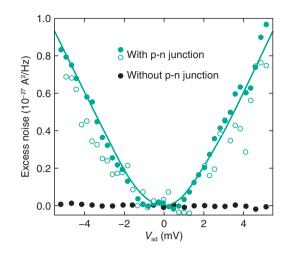
Fig. 3. Shot noise generated by p-n junction as a function of the bias applied to the electron channel  $V_{sd}$ . Solid cyan and black circles represent the measured noise in the presence and absence of p-n junctions. Open cyan circles represent the noise in the presence of a p-n junction obtained by applying bias to the hole channel.
