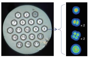
Six modes can propagate within each core.
