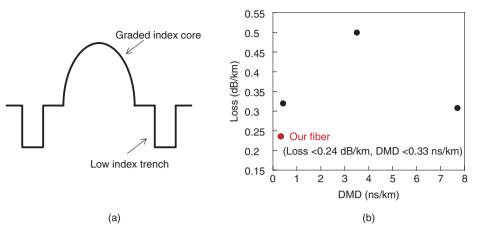
Fig. 7. (a) Schematic diagram of trench assisted graded-index core profile, (b) transmission loss vs. DMD of recently reported few-mode multi-core fibers.
