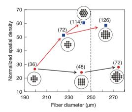
Fig. 6. Relationship between spatial density and fiber diameter of various multi-mode multi-core structures.
