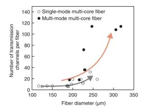
Fig. 3. Relationship between transmission channels per fiber and fiber diameter.
