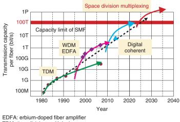
TDM: time division multiplexing WDM: wavelength division multiplexing
