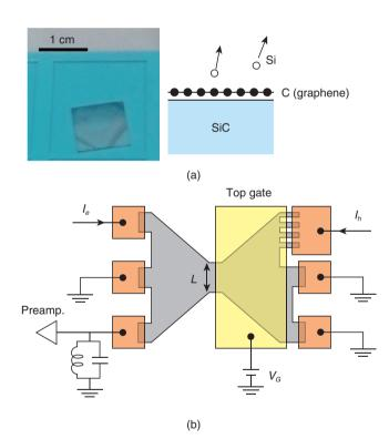
Fig. 2. ((a) left) Photograph of graphene grown on SiC. ((a) right) Schematic of graphene growth on SiC. (b) Device structure of graphene with a p-n junction. Gray region represents n-doped graphene. Tuning the bias of the top gate (yellow region) changes the carrier type in the gated region to a hole, and a p-n junction is formed at the interface between the gated and ungated regions. Orange regions are ohmic contacts.
