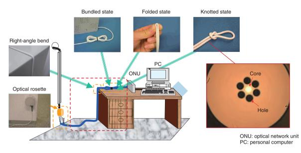
Free-bending optical cord achieves optical communications in a bent, bundled, folded, or knotted state. Enables do-it-yourself optical wiring in a similar way to electrical wiring
