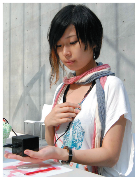
Fig. 2. Feeling your own heartbeat through the vibrations of a box (heartbeat box) in the palm of your hand.
