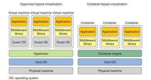
Fig. 3. Schematic of hypervisor-based virtualization and container-based virtualization.
