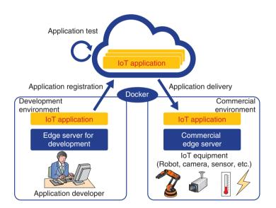
Fig. 5. Schematic of development, delivery, and management of IoT application based on Docker.
