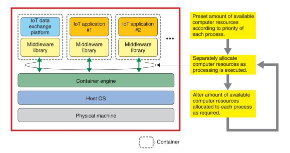
Fig. 4. Schematic of edge server using container-based virtualization.
