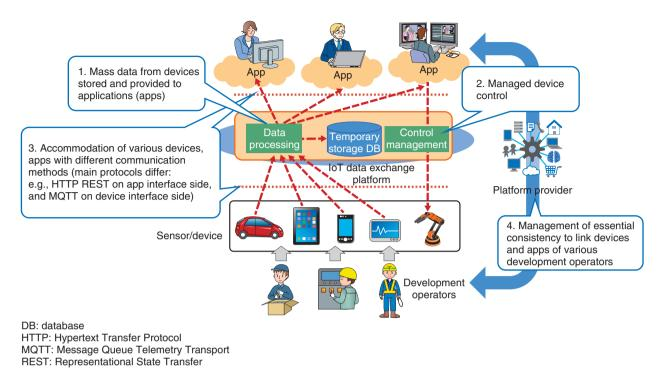
Fig. 1. IoT data exchange platform.
