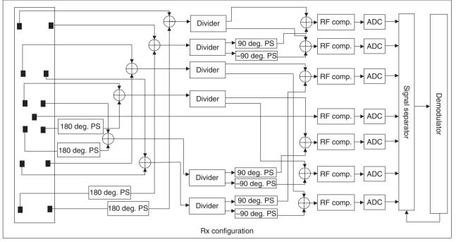
ADC: analog-to-digital converter RF comp.: radio frequency components PS: phase shifter
