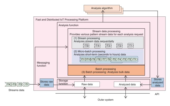
Fig. 5. Outline of Fast and Distributed IoT Processing Platform.
