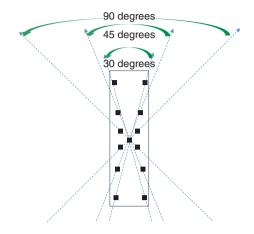
Fig. 4. Proposed Rx antenna.
