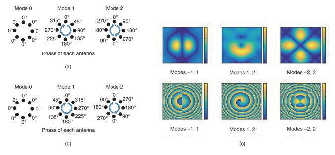
Fig. 2. (a) Generation of OAM modes with a UCA, (b) separation of OAM modes with a UCA, and (c) intensity distribution (above) and phase distribution (below) of combined OAM modes.
