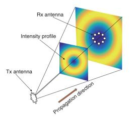
Fig. 3. Conceptual drawing of OAM beam divergence.
