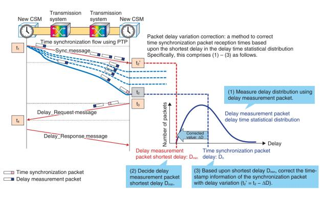
Fig. 4. Packet delay variation correction method.
