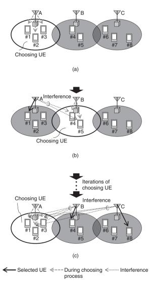
Fig. 2. Procedure for deciding the combination in the search process.
