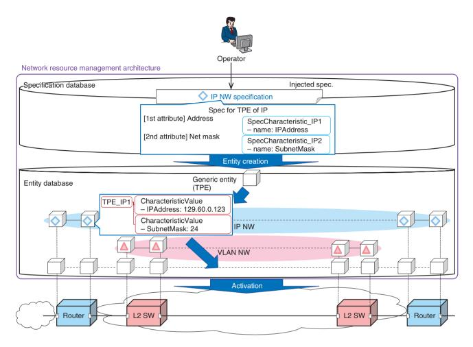
Fig. 5. Example of IP network.
