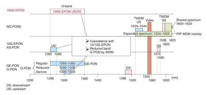
Fig. 3. A wavelength plan for 100G-EPON.
