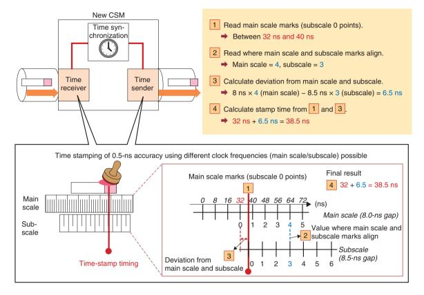
Fig. 3. Time stamping using Vernier scale.
