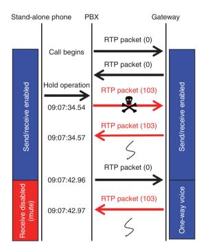
Fig. 2. Results of RTP packet analysis.
