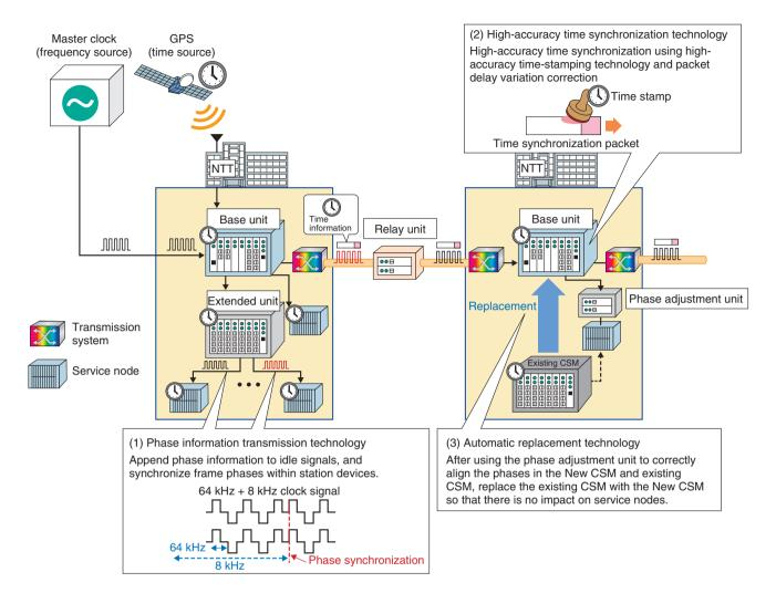
Fig. 2. New CSM configuration.
