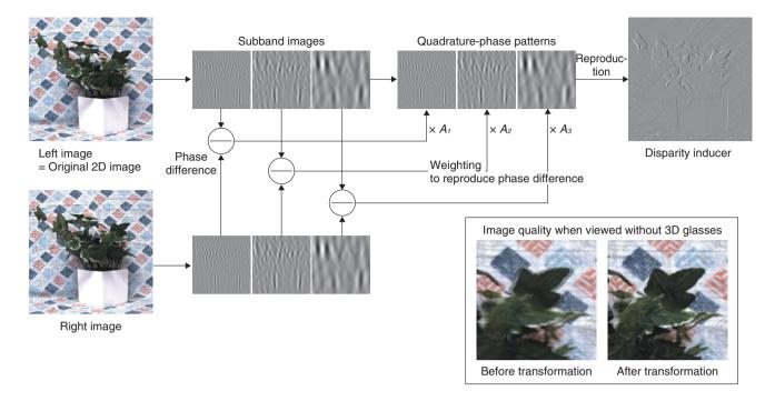
Fig. 4. Process overview to generate a disparity inducer from a standard stereo pair.
