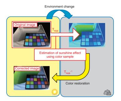
Fig. 5. RGB information correction using a color sample board.
