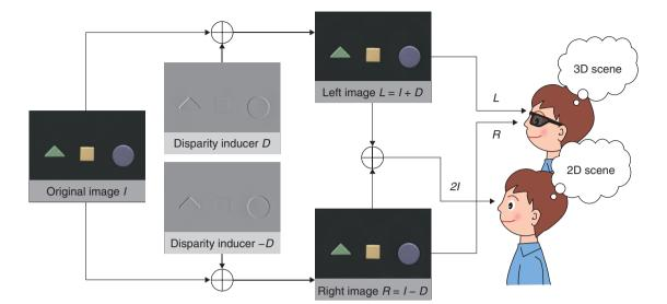
Fig. 1. Schematic of how our method cancels stereo ghosts for viewers without 3D glasses.
