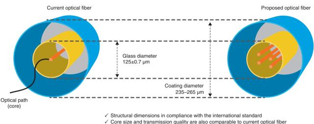
Fig. 1. Features of proposed multi-core fiber.
