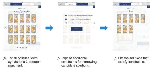
Fig. 4. Demonstration system for designing layouts of an apartment.
