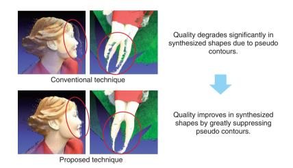
Fig. 5. Comparison of results applying depth-image rectification techniques.
