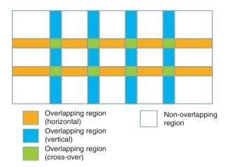
Fig. 2. Example of the overlapping regions used in  $5(H) \times 3(V)$  4K video stitching.
