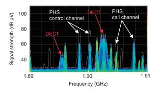
Fig. 4. Radio signal environment (measurement point A).
