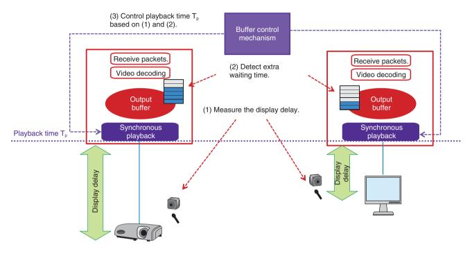
Fig. 6. Controlling the playback buffer region.
