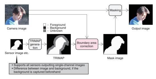
Fig. 1. Object extraction process.
