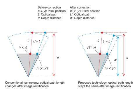
Fig. 3. Conceptual diagram of depth-image correction technology.
