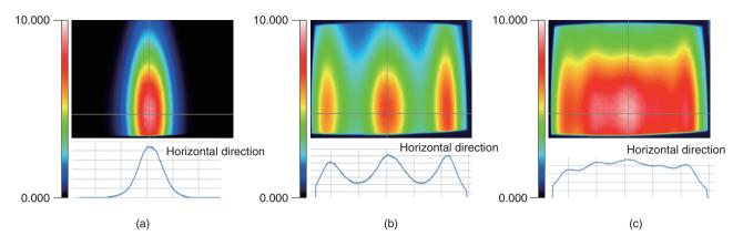
Fig. 5. Luminance distribution of obtained spatially imaged iris plane.
