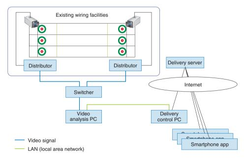
Fig. 4. Configuration of curling-stone location delivery system.
