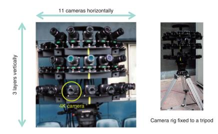
Fig. 4. Video camera rig with multiple 4K cameras mounted horizontally and vertically.
