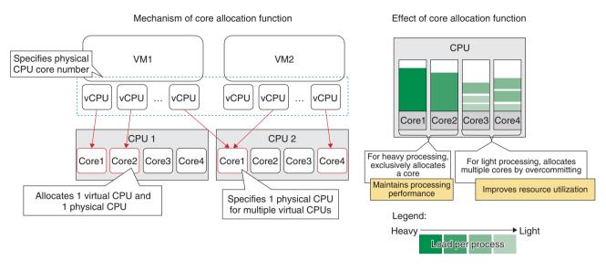
Fig. 3. CPU-core allocation function.
