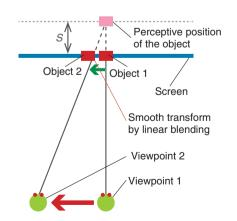
Fig. 3. Depth perception by motion parallax.
