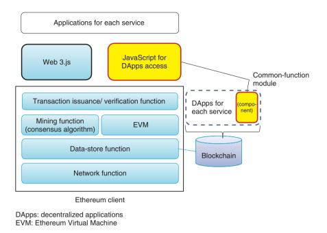
Fig. 2. Proposed module for managing authority and concealing data used in developing blockchain applications.
