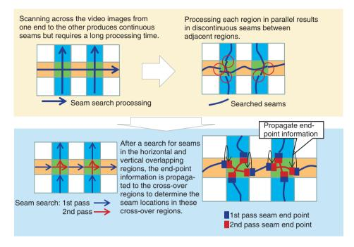
Fig. 3. Parallel processing to ensure seam continuity.
