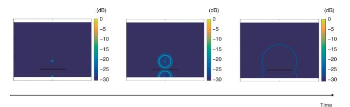
Fig. 3. Wave front of monopole sound source.
