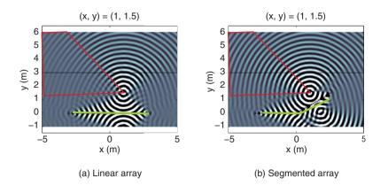
Fig. 5. Extended sweet spot. The area within the red border in (b) shows that the radiated sound from the focused source is stronger than the corresponding area in (a). This means that a larger area of the desired sound field is reproduced by a segmented array than by a linear array.
