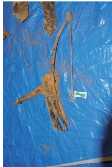
Fig. 4. Photo of buried anchor showing considerable deterioration.
