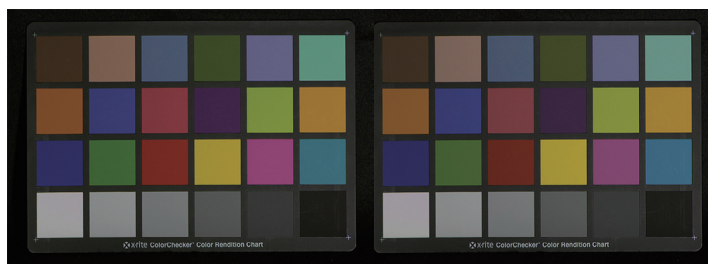
Fig. 4. Captured images of color chart under synthesized daylight (left) and under the designed illumination (right).
